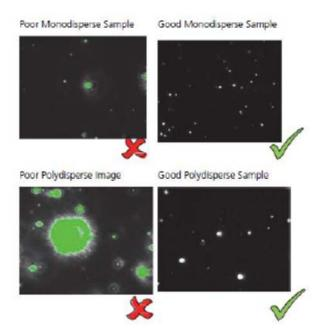
14. Initial focus is set with the manual control on the side of the NanoSight NS300, adjust for fine focus within the software Indistinct particles, as in a) will give inaccurate results. Ideally, particles should appear as in b) but those in c) will be acceptable if that is the best image that can be achieved.
