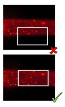
13. Correctly setting up the camera and sample image prior to capturing the video are essential to achieving valid results. Increase the Camera Level until all of the particles in the sample can be seen clearly but no more than 20% are saturated (colored pixels).
