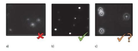
15. Concentration. The instrument can work with particle concentrations in the range of  $\sim 10^6$ -  $10^9$  particles/ml, which is approximately 20-100 particles in the field of view. Too high a sample concentration may prevent accurate particle tracking. Lower concentrations require longer capture and analysis time to produce statistically significant results. Using the NanoSight syringe pump will improve results by sampling more particles.
